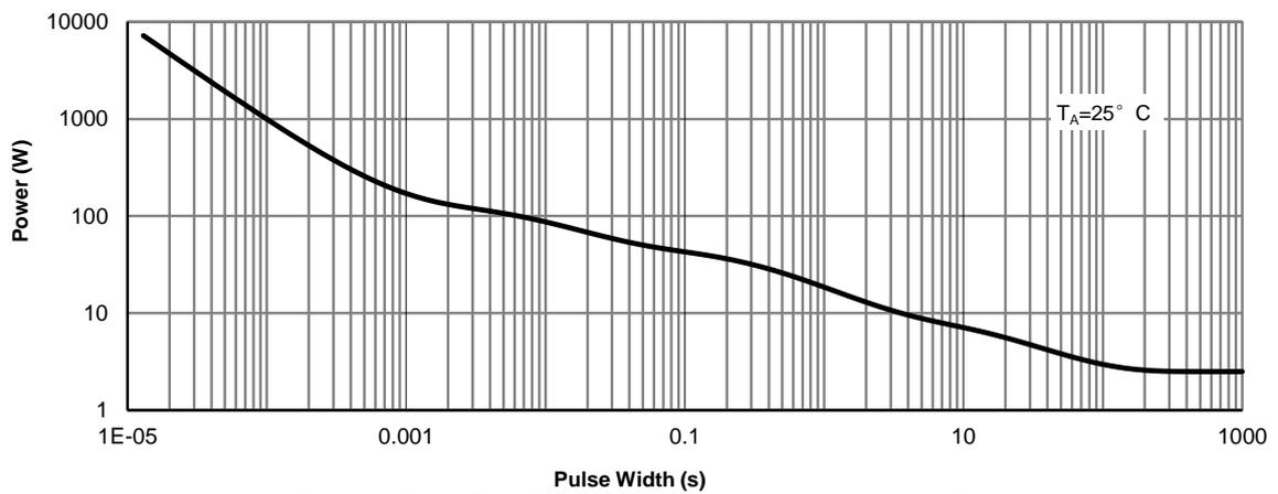
Figure 14: Single Pulse Power Rating Junction-to-Ambient (Note H)
