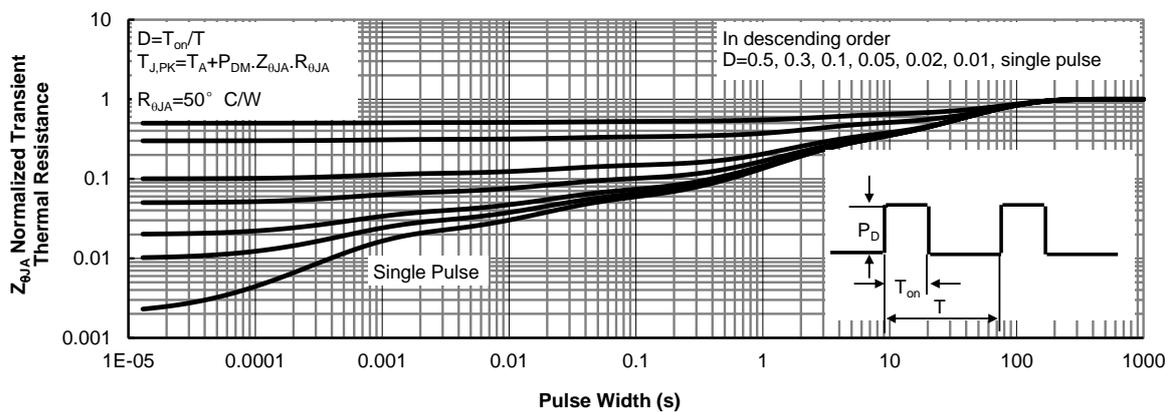
Figure 15: Normalized Maximum Transient Thermal Impedance (Note H)
