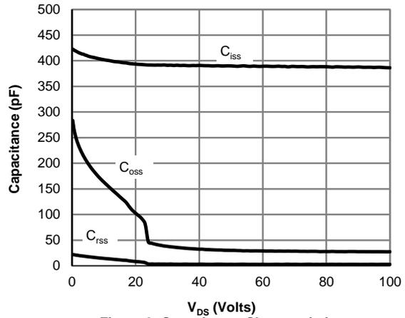
**Figure 8: Capacitance Characteristics**
