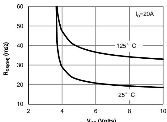
**Figure 5: On-Resistance vs. Gate-Source Voltage (Note E)**
