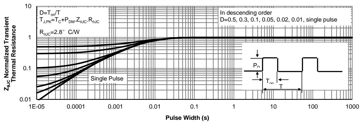
**Figure 11: Normalized Maximum Transient Thermal Impedance (Note F)**
