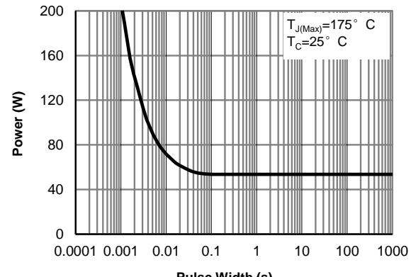
**Figure 10: Single Pulse Power Rating Junction-to-Case (Note F)**
