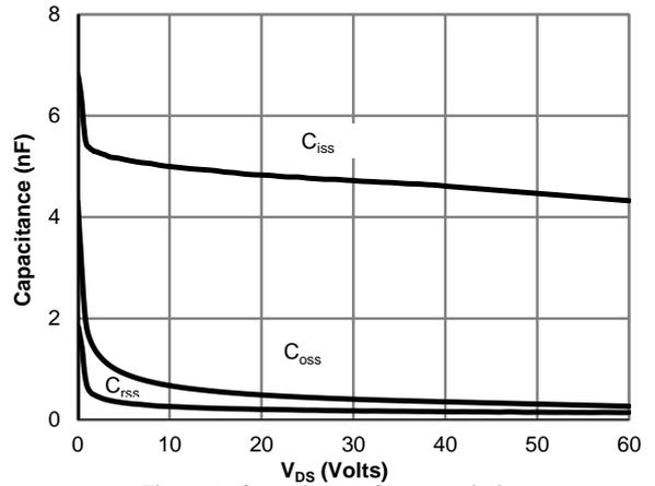
**Figure 8: Capacitance Characteristics**
