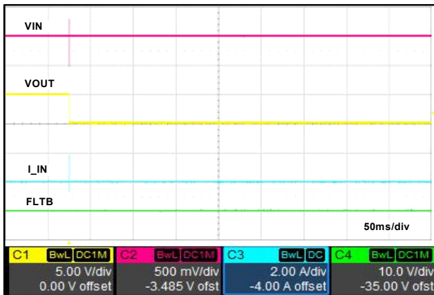
Figure 15. Short Circuit Protection (No Load, Device Option -04)
